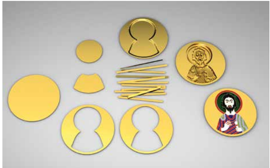
Figure 1.23 Drawing showing how a piece of gold, perhaps a coin, might be divided effectively to construct a Middle Byzantine enameled medallion.
