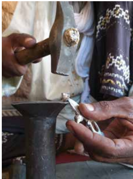
Kammo forges each of the cones against the edge of his anvil.
