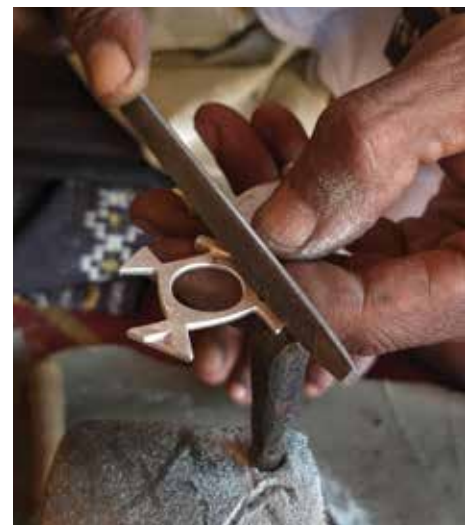
Using a graver made from a small screwdriver, the surface is engraved with traditional patterns.
