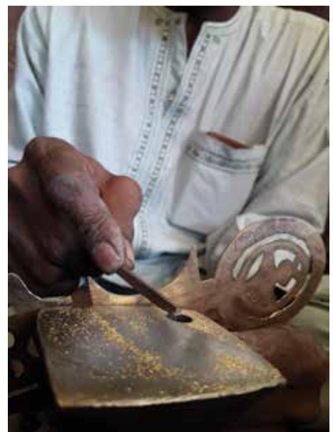
Scoring, chiseling and filing to refine the design.
