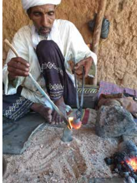
Kammo steadies the crucible against a wooden rod and pours molten silver into the mold.
