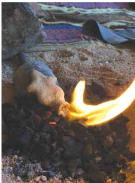
The mold is set onto hot coals to burn out the wax. Most will be poured out and reused.
