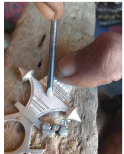
Using a graver made from a small screwdriver, the surface is engraved with traditional patterns.
