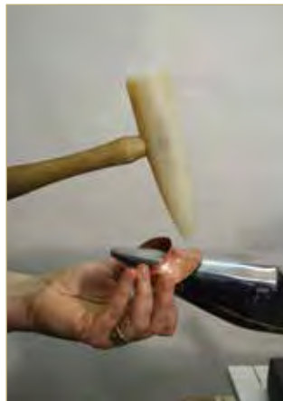
Bouging on a sinusoidal stake... ... and the horn of an anvil.
