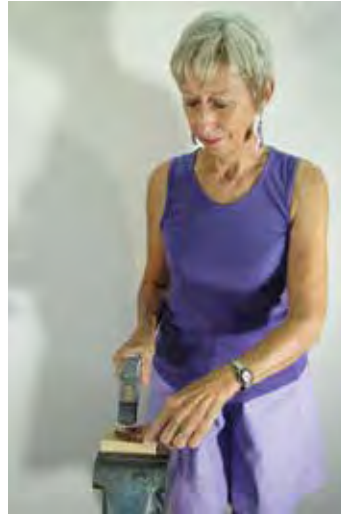
Betty Helen demonstrates the proper stance. Notice how her right shoulder, elbow, and wrist are in line with the work. The proper grip on the hammer is relaxed, with fingers and thumb comfortably encircling the handle.
