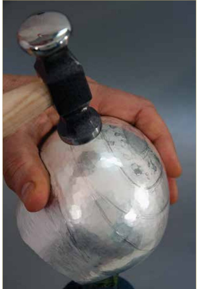
The checkerboard technique refers to a pattern of blows separated by unstruck areas. This strengthens and stabilizes the form.
