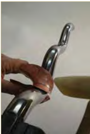
Bouging on a sinusoidal stake... ... and the horn of an anvil.
