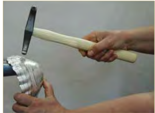
Betty Helen demonstrates the proper stance. Notice how her right shoulder, elbow, and wrist are in line with the work. The proper grip on the hammer is relaxed, with fingers and thumb comfortably encircling the handle.
