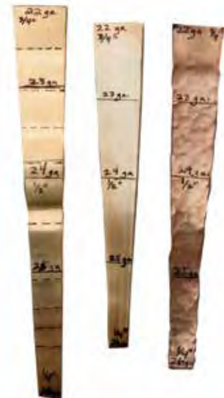
Center: the initial blank. The strip on the left was rolled and planished. The strip on the right was thinned by planishing alone.
