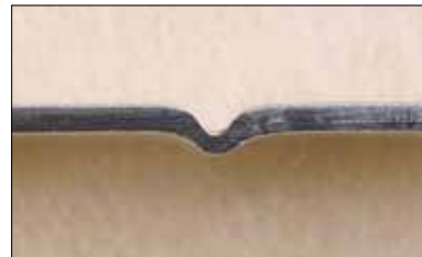
The profile shot shows a cross-section of the groove made by a liner.
