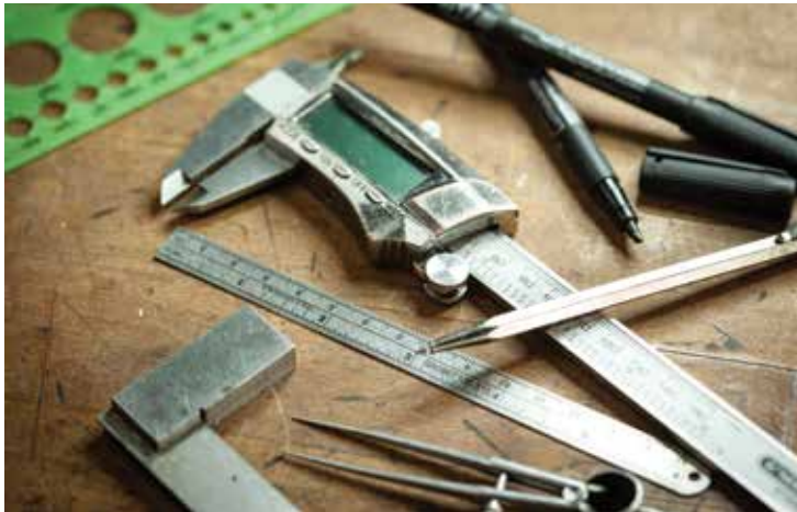
Caliper, ruler, compass, square, dividers, permanent markers and scriber.
