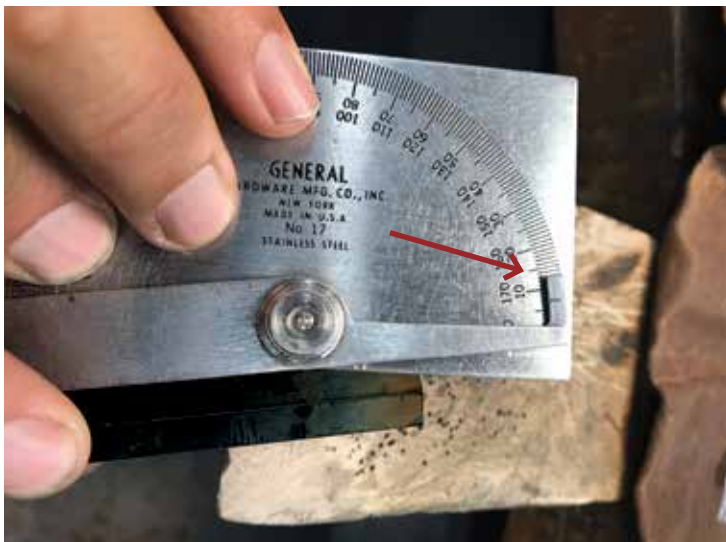
An angle gauge like this is useful to determine precise angles, for instance on the end of the tool. This photo shows that the slope on the tool is at 12° from the vertical axis, shown at the arrow.
