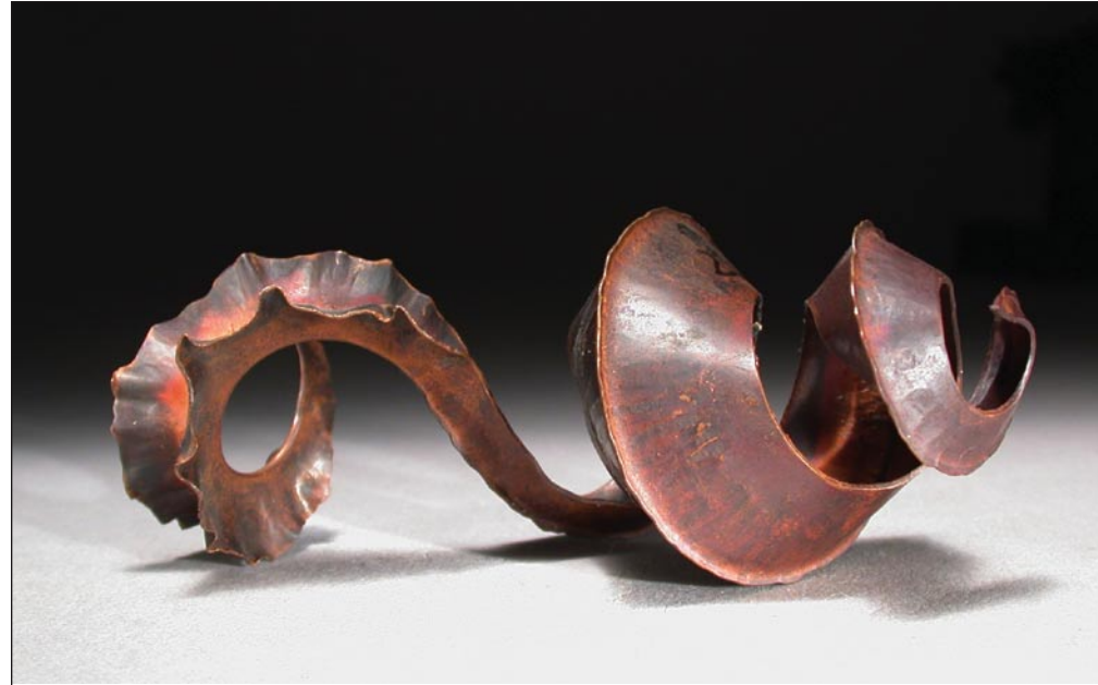
This shape was made with a combination of forged line-folds, one section forged on the open side and the other on the closed sides. In addition to demonstrating what a big difference this simple variable can make, this piece shows the value of combining different types of foldforming.
