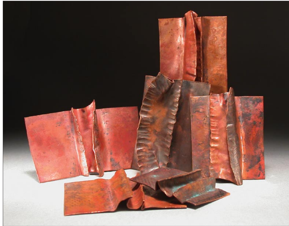
T-Folds. Primary variables are achieved by whether the fold edges are forged and how the sheet is unfolded.
