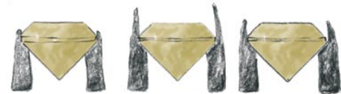
If the bezel wall is too short (left), the stone may fall out. If the bezel is too tall (center), it will be difficult to press down, and it will cover the stone. The goal (right) is a bezel that will cover about a third of the crown after firing.
