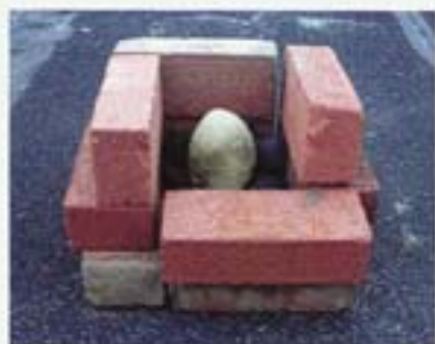
When the miso-yaki coating is dry, build a kiln around the work with fire bricks.
