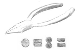
The shapes show the cross sections of the most popular pliers: chain-nose, flat, round-nose, and ring forming.
