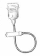
A flex-shaft is used for drilling, grinding, and polishing.
