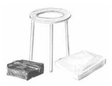
Three time-tested soldering surfaces are a charcoal block, a soft firebrick, and a steel tripod, usually used with a screen on top.
