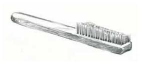
Whether steel or brass, lubricate the burnishing action with soap and water.
