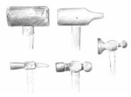
Here are some of the most common hammers and mallets. From the top: rawhide, plastic, chasing, ball-peen, and rivet.
