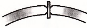
Figure P.10. A platinum ring, ready for welding with a small sliver of the same metal held by tension between the beveled corners at the seam
