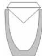
After moving the prongs inward, the stone sits on top as it should, covering half of each prong when viewed from above.
