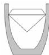
The opening in this setting is too large; the stone drops in.
