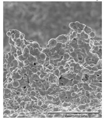
This image was taken by a scanning electron microscope, and shows properly sintered PMC at a magnification of 1000 times actual size. The individual silver particles have fused together to form solid metal.
