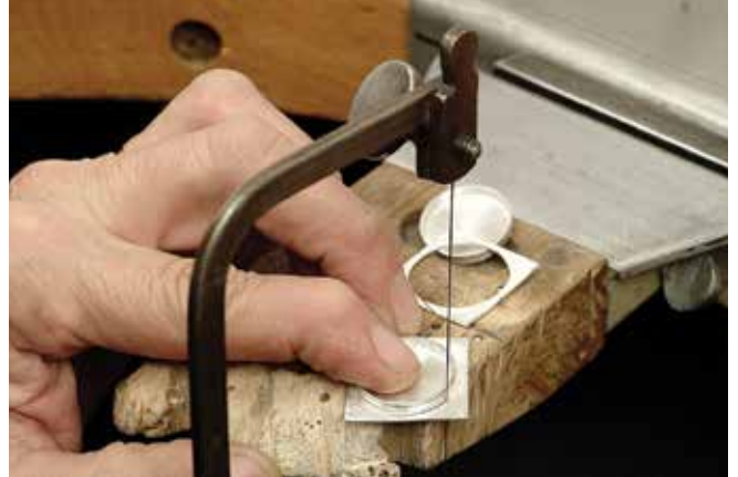
Figure 19.10 Sawing off the excess.
