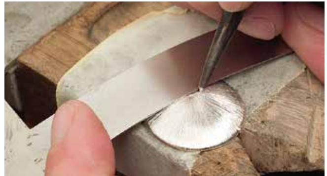
Figure 19.28 Adding a radial texture.
