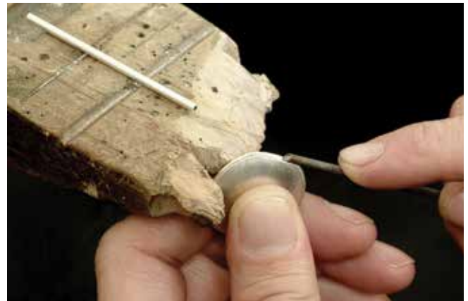
Figure 19.19 Filing a cradle for the hinge.
