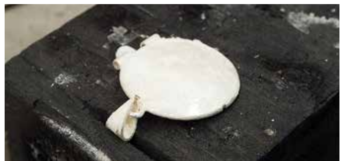
Figure 19.26 Soldering the bail in place.
