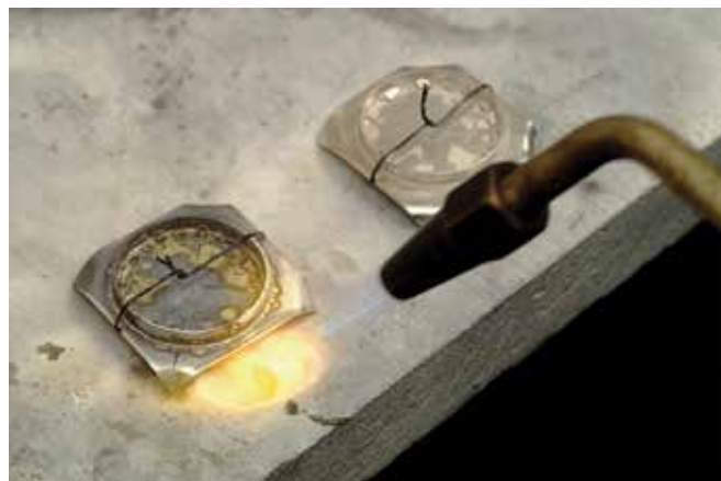
Figure 19.9 Soldering bezels to sheet (note that fire coat has been omitted from the photo for clarity).
