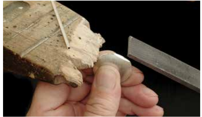
Figure 19.18 With halves glued together, file a flat spot for the hinge.
