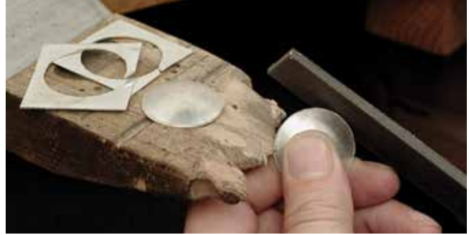
Figure 19.14 Filing the domed halves.
