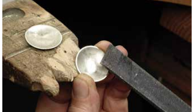
Figure 19.4 Filing the rims flat.
