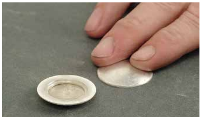
Figure 19.17 Sanding the interiors.
