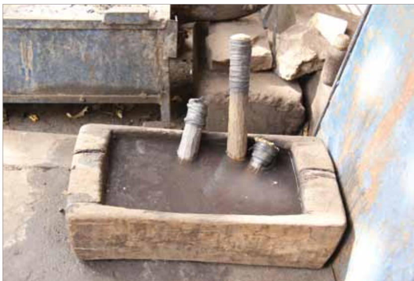
Forging hammer left all night in water so the wood swells up and holds the head for a day of work. Bamako, Mali.
