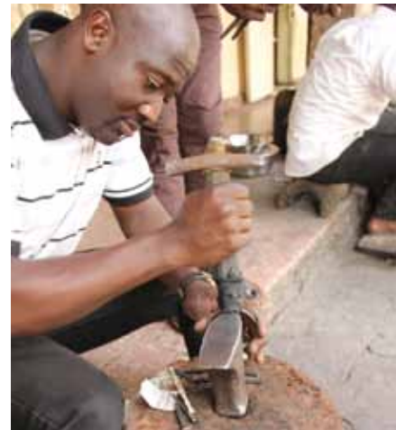
Modibo uses the wooden handle on the horn of the anvil to smooth the curve.
