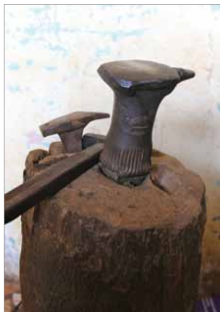
Fulani anvil made from a truck axle. A small Toucouleur anvil. Conakry, Guinea.
