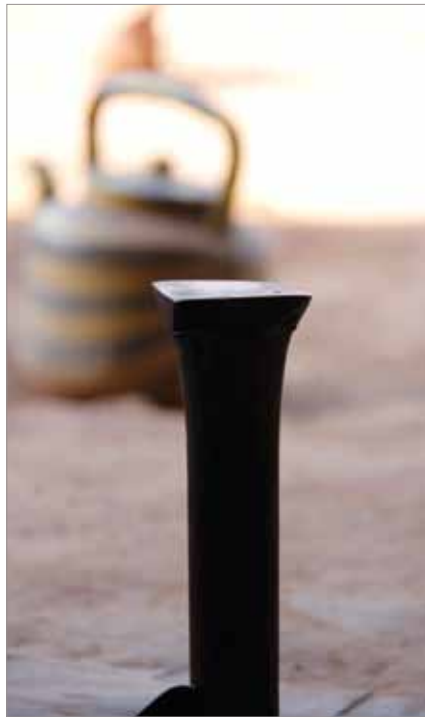
Tuareg anvils. A piece of rubber, leather or canvas is set around the base of the anvil to catch metal filings.
