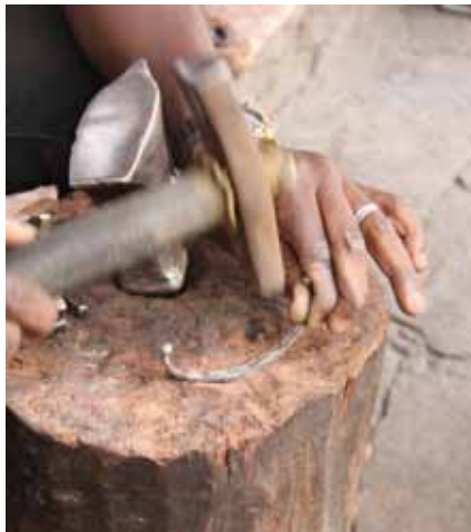
The bending process continues, working from the center outward.
