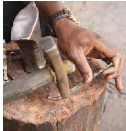
To bend the bracelet, Modibo uses an indentation on his stump.
