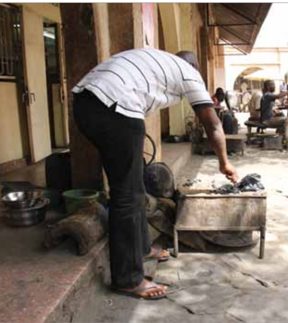
Annealing on the forge.
