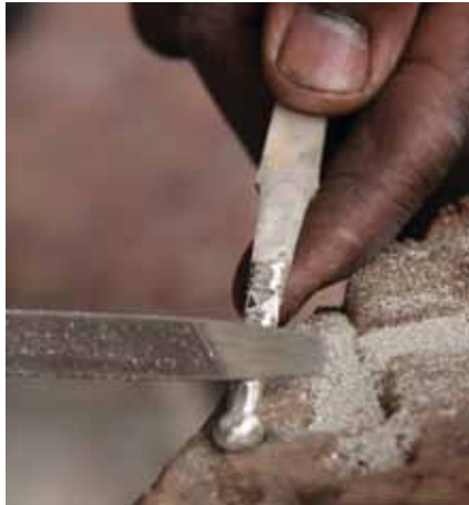
The round shank of the bracelet is filed to create a design.
