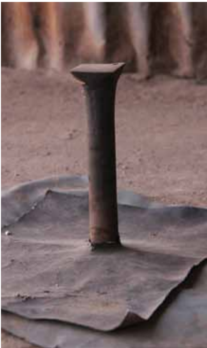
Tuareg anvils. A piece of rubber, leather or canvas is set around the base of the anvil to catch metal filings.
