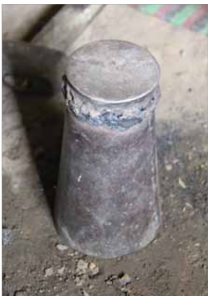
Anvil of repurposed steel part, Bamako, Mali.
