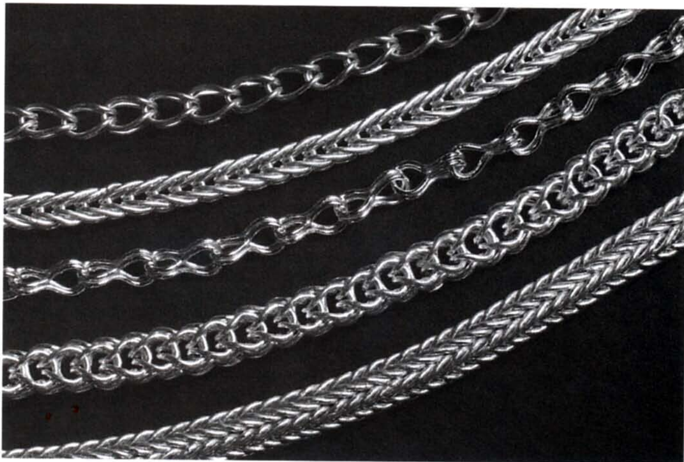
FIGURE 1.1 Basic Loop-in-Loop Chain Types (from top to bottom): Single, Double, Pinched Loop, Two-Way Single, Two-Way Double.
