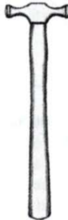
FIGURE 2.10 Small planishing hammer
